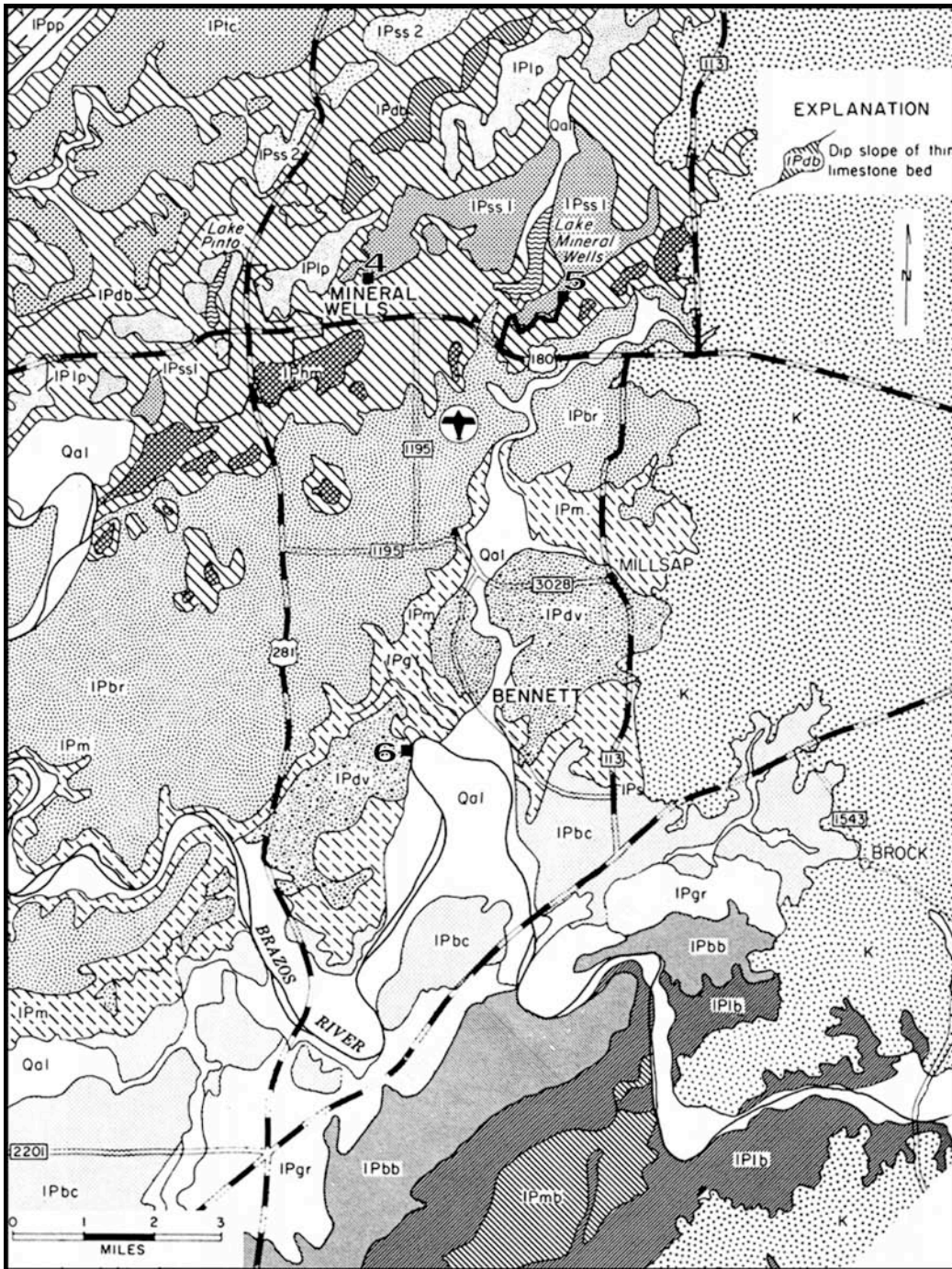
Figure 10. Geologic map of the Mineral Wells area showing steps 4, 5 and 6. Step 4 is within the Mingus Formation. Step 5 represents a window into the underlying Brazos River Formation fluvial conglomerates at Mineral Wells State Park. Step 6 is within the Dobbs Valley sandstone of the Mingus Formation, Strawn Group (modified after Brown et al., 1973).
